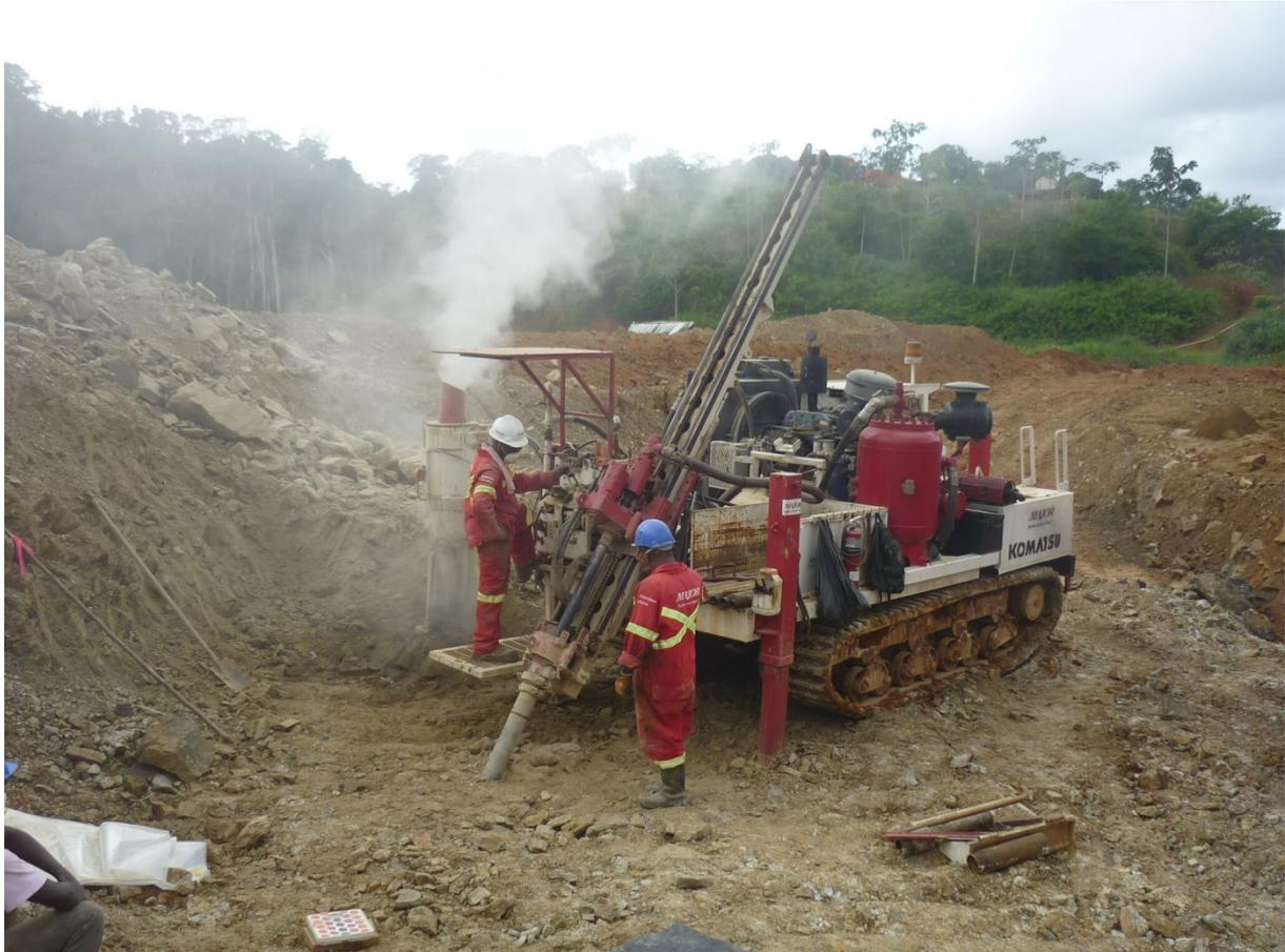
**Figure 1: 2013 RC drill rig (Komatsu) - Yaou gold project**
