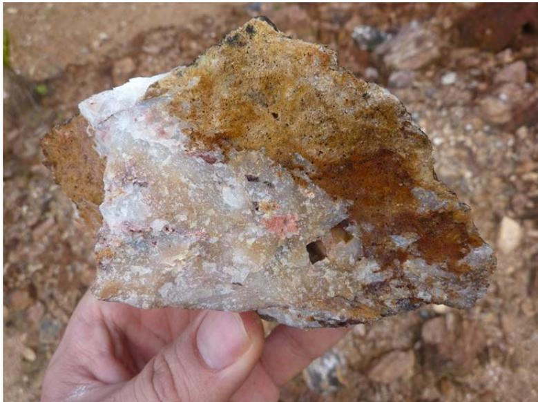
***Photo 15: Hand specimen of quartz veining with cubic pyrite boxwork***
