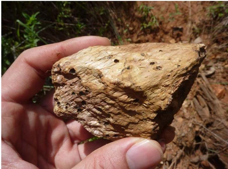
***Photo 17: Weathered schist with frequent oxidized pyrite***
