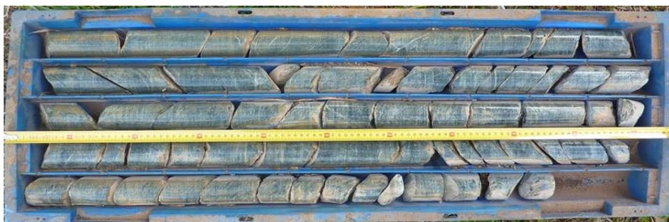
**Figure 8: Drill core box – BRGM2NQ type**
