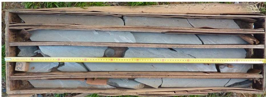
**Figure 7: Drill core box – BRGM1NQ type**
