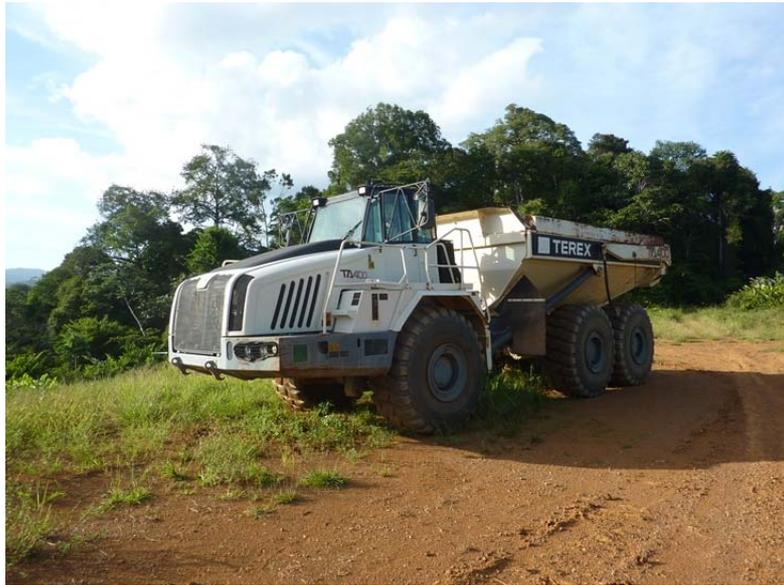
*Photo 7: Articulated mining truck (TEREX TA400 - 40 t)*
