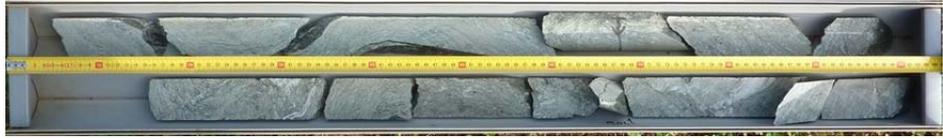
**Figure 12: Drill core box – AUP1HQ type**
