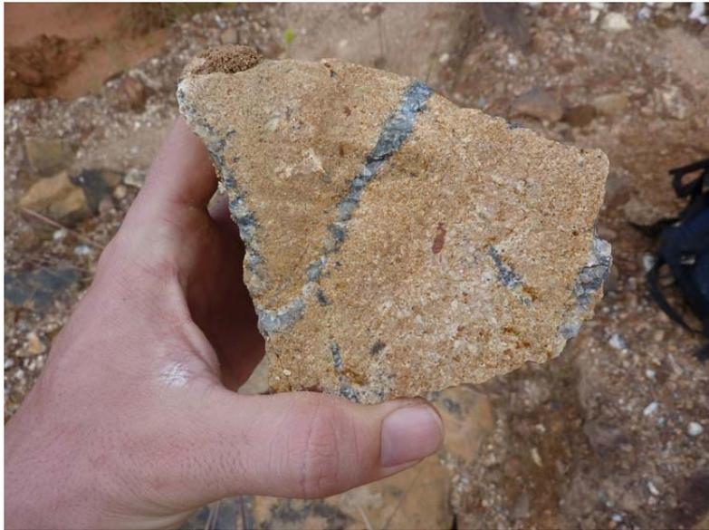
*Photo 12: Hand specimen of felsic dyke (mineralization host)*
