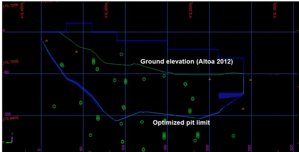
Figure 22: Zone A recommended drilling pierce point locations (orange triangles)
