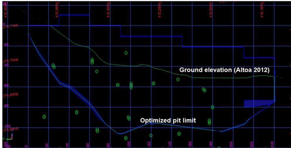
**Figure 13: Zone A resource shell and optimised pit section with pierce points of drillholes**
