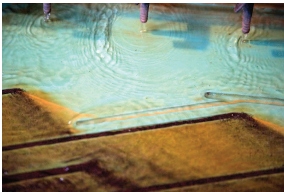
A stream of gold particles flowing down the grooves of a vibrating table in the final stages of one of Auplata's gravity separation circuits in French Guiana. Auplata is one of the biggest private-sector employers in the department.
